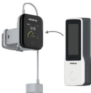
3. Check the screen of the EP30 monitor immediately. If a confirmation screen is displayed, press the touch button to confirm the pairing. Failing to do so would cancel the pairing.
