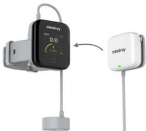
4. Check the screen of the EP30 monitor immediately. If a confirmation screen is displayed, press the touch button to confirm the pairing. Failing to do so would cancel the pairing.
