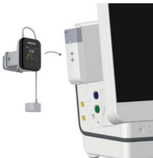
3. Check the screen of the EP30 monitor immediately. If a confirmation screen is displayed, press the touch button to confirm the pairing. Failing to do so would cancel the pairing.
