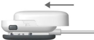
3. Place the front of the ECG module close to the screen of the EP30 monitor until you hear a beep.
