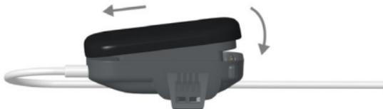
2. Put the ES30 ECG unit onto the connector of the ES30 docking with both sides aligned. Then slide the ES30 ECG unit up as indicated below until the two click into place.
