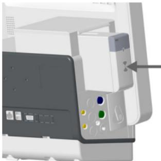
2. Place the EP30 monitor close to the pairing area of the receiver until you hear a beep.
